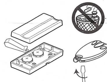
To replace cover, snap shut along both sides. The lithium batteries should produce power for up to 5 years. To replace batteries, use a coin, the visor clip or screwdriver blade to pry open the case, as shown ("Open" location is stamped on back.)
