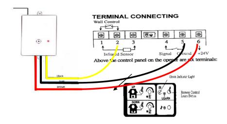
The receiver goes to terminals 2 (Wall Control), 5 (GND), 6 (+24V).
